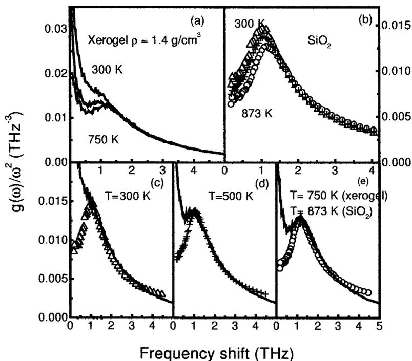
Figure 4. Neutron spectral intensity: (a) on xerogel with  $\rho = 1.4 \text{ g cm}^{-3}$  at 300 K, 500 K, and 750 K; (b) on vitreous silica at 300 K, 500 K, and 873 K; (c, d, e) on xerogel with  $\rho = 1.4 \text{ g cm}^{-3}$  and vitreous silica at different temperatures.
