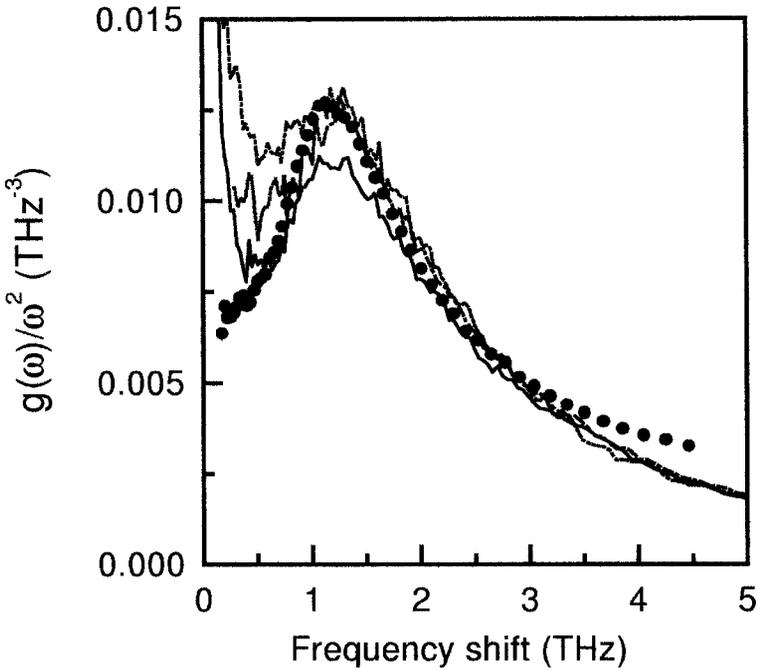
Figure 5. Neutron spectral intensity for xerogels at 750 K, with  $\rho = 0.8 \text{ g cm}^{-3}$  (full line),  $\rho = 1.4 \text{ g cm}^{-3}$  (dot-dashed line),  $\rho = 1.73 \text{ g cm}^{-3}$  (dotted line), and for vitreous silica at 873 K,  $\rho = 2.2 \text{ g cm}^{-3}$  (circles). Neutron data on vitreous silica are from Wischnewski *et al.* (1998).
