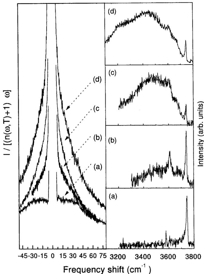
Figure 2. Raman spectral intensity at room temperature for the xerogel with  $\rho = 1.73 \text{ g cm}^{-3}$ : (a) after annealing at 750 K; (b) after ageing for 4 h; (c) after ageing for 24 h (this measure was at 400 K); and (d) after ageing for 48 h.
