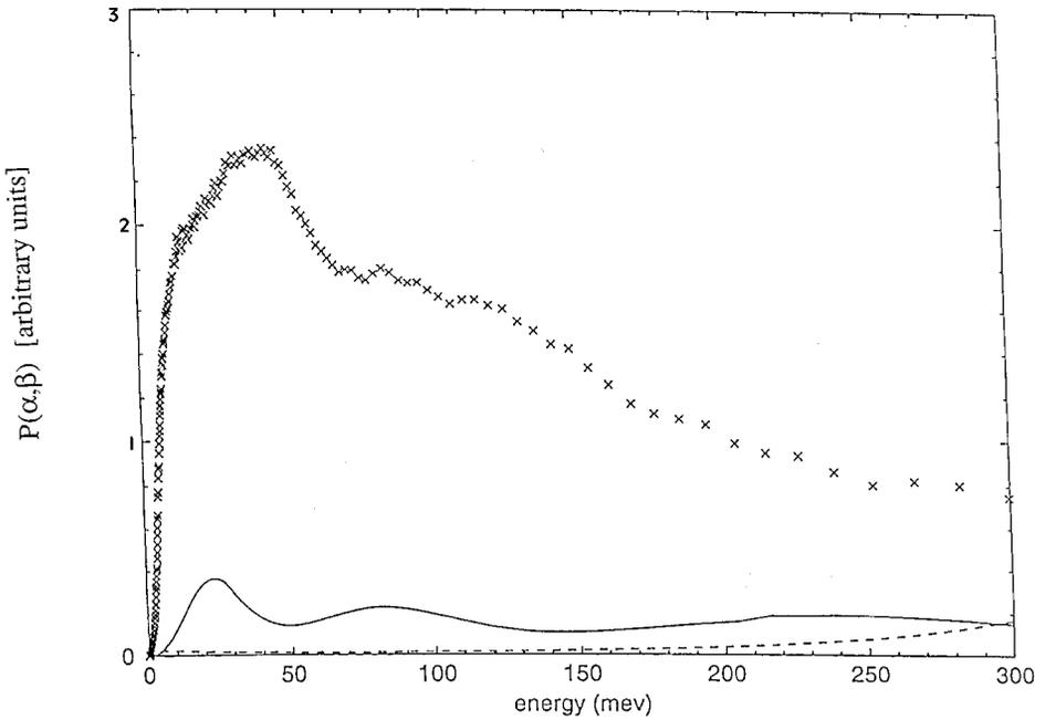
Figure 1. Experimental  $P(\alpha, \beta)$  (crosses) at 750 K for the xerogel with  $\rho = 1.4 \text{ g cm}^{-3}$ , with the multiphonon (continuous line) and background (broken line) contributions.
