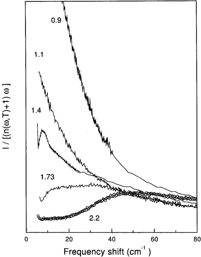
Figure 3. Raman spectral intensity at 750 K on xerogels with  $\rho = 0.9 \text{ g cm}^{-3}$ ,  $\rho = 1.1 \text{ g cm}^{-3}$ ,  $\rho = 1.4 \text{ g cm}^{-3}$ ,  $\rho = 1.73 \text{ g cm}^{-3}$ , and  $\rho = 2.2 \text{ g cm}^{-3}$  (melt quenched vitreous silica).
